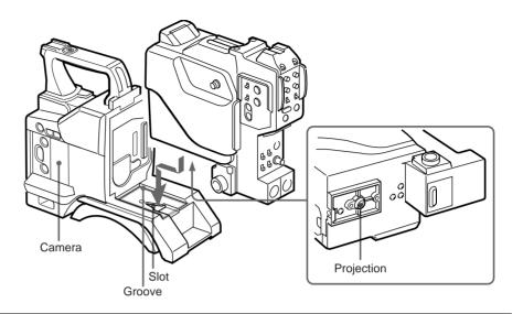
3 Slide the unit along the groove on the camera, and press firmly until fixed.
